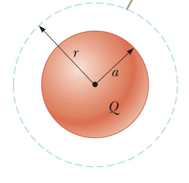
Spherical symmetry means the Gaussian surface must be spherical
